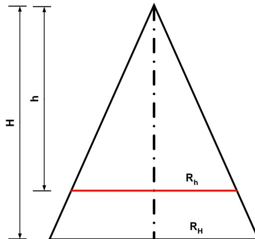
$$V_H = \frac{1}{3}\pi R_H^2 H; V_h = \frac{1}{3}\pi R_h^2 h, \text{ or } \frac{R_h}{h} = \frac{R_H}{H} \text{ et } V_H = 2V_h \Rightarrow \frac{1}{6}\pi R_H^2 H = \frac{1}{3}\pi \frac{R_H^2}{H^2} h^3$$
