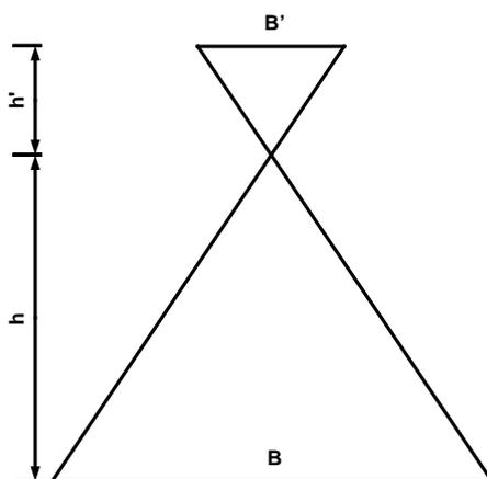
$$\text{On a : } \left(\frac{h'}{h}\right)^2 = \frac{B'}{B} \Rightarrow h = h' \cdot \sqrt{\frac{B}{B'}} \Rightarrow \Delta h = |h' - h| = \left| h' - h' \cdot \sqrt{\frac{B}{B'}} \right| = h' \left| 1 - \sqrt{\frac{B}{B'}} \right| \Rightarrow h' = \frac{\Delta h}{\left| 1 - \sqrt{\frac{B}{B'}} \right|} \quad (1)$$
